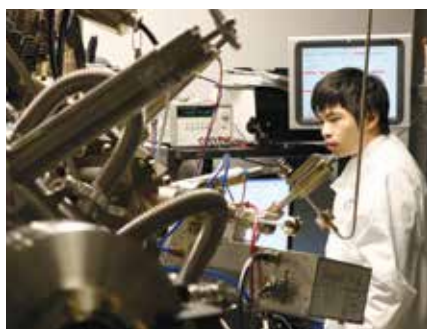
Xianhe Liu sets up the molecular beam epitaxy system to grow deep UV LEDs.
