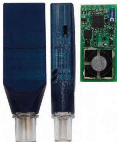
The smartphone-based CO detector, with views from the front, side, and of the internal circuit board.
