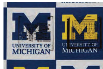
Thin film transistors (left) and Schottky diodes (right) made in Prof. Becky Peterson's lab using amorphous Zn-Sn-O semiconductor layers.
